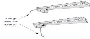
NOTE!: To connect the mains use only approved cable joiner suitable for outdoor applications.
