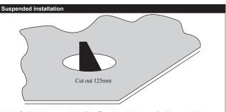
1.1.1. Cut hole in suspended ceiling. The aloved thickness of ceiling material is max.
