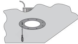
1.1.3. Fit the decoration ring with screws in the suspended ceiling.
