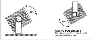
Unfix by hand the screw and aim the fixture to the wish position and fix.
