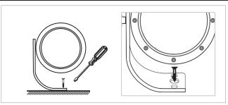
Screw the fixture to the surface (M12 or 2xM10)
